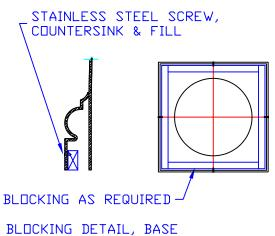
CAPITAL & BASE SEPARATE ALL COLUMNS SHIPPED IN HALF-UNITS COLUMN WILL FIT UP TO: 6" SQ. BEAM Ø9" COLUMN
