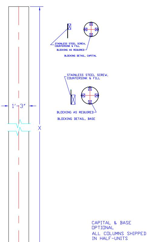
COLUMN WILL FIT UP TO: 10" SQ. BEAM Ø14" COLUMN
