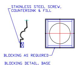
CAPITAL & BASE ATTACHED ALL COLUMNS SHIPPED IN HALF-UNITS COLUMN WILL FIT UP TO: 12" SQ. BEAM Ø17" COLUMN
